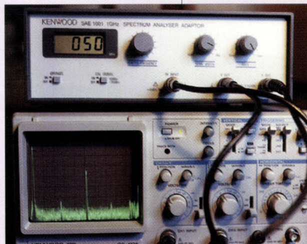
Fig. 3: The CS-4125 and the SAE-1001 partnership in action in Gordon King's laboratory, the display showing a 50MHz signal at about -35dBm with sidebands either side at around -65dBm. The group of responses at the extreme right are local Band II f.m. signals! The left hand response represents the start at zero frequency.
