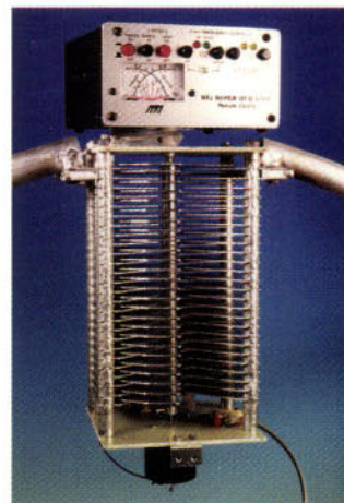
The enormous butterfly capacitor on the MFJ-188 Loop Antenna.
